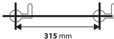
3. Use a drill to drill the mounting holes. Use a 6 mm drill bit for drilling. The depth of the holes must be at least 26 mm deep. Do not use a smaller size!
